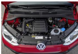
The 85kW / 115PS 1.0 TSI in the up! GTI
