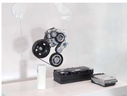
48-V belt-integrated starter generator, 48-V battery and DC/DC converter
